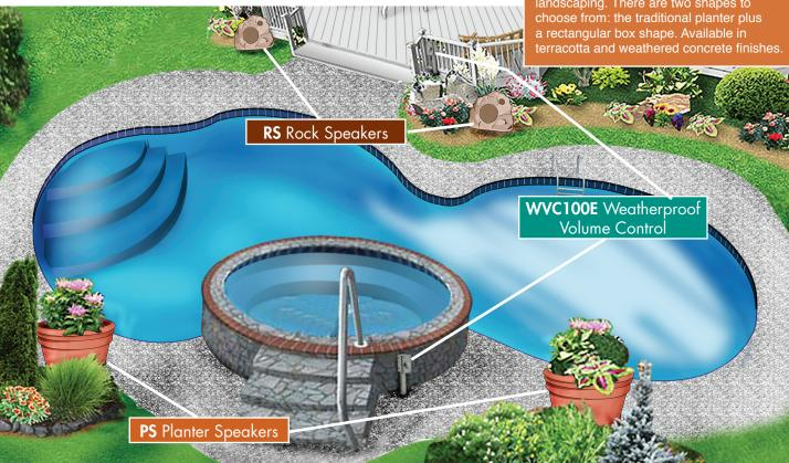
Individual zone volume controls are the best solution for large, single zone outdoor areas with multiple listening areas. In this illustration, Niles WMVC100E Weatherproof Muting Stereo Volume Controls are positioned for easy access near the hot tub and the deck. To adequately power all these loudspeakers, a Niles SI-1260 12-Channel Systems Integration
